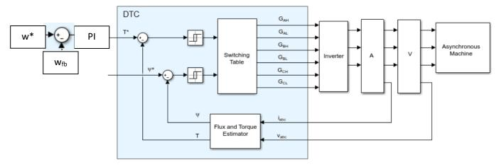
$$\Psi_{\alpha} = (v_{\alpha} - i_{\alpha} R_s) \frac{T_s z}{z - 1}$$
