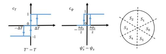
Assume the reference value of flux to be at the rated value,  $\psi_s^*$  of 1.25 Wb, and *flux error* band of  $\pm 10\%$  for the hysteresis comparator of flux.
