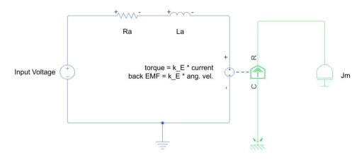
Assume that the electrical parameters of the motor are  $R_a = 0.12$  ohms,  $L_a = 0.0012$  H,  $k_E = 0.2$  units, and the motor's rotor has a moment of inertia  $J_m = 0.25$  kg m<sup>2</sup>.
