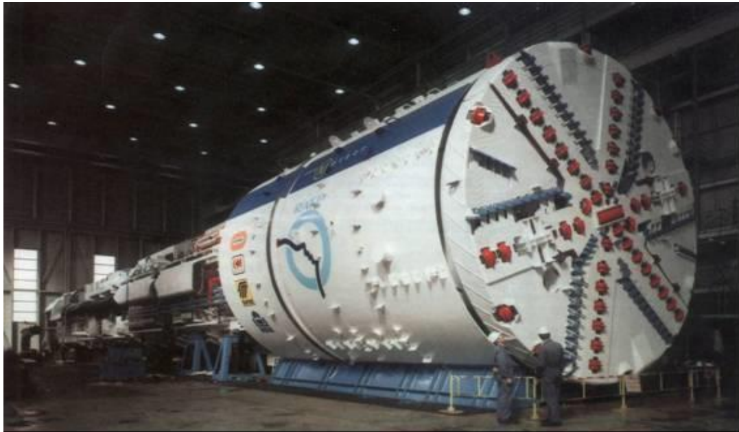
FIGURE 5.46: EARTH PRESSURE BALANCE TBM
