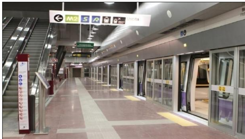
FIGURE 9.5: PLATFORM SCREEN DOOR
