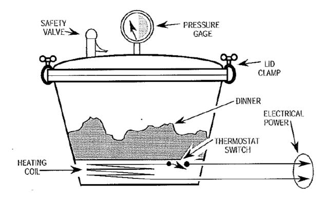
Operator's Tasks: (1) loads cooker, (2) closes/seals lid, (3) connects power, (4) observes pressure, (5) times cooking at prescribed pressure, (6) offloads cooked food.
