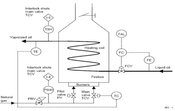
The oil flow is controlled by a flow control set which includes:
