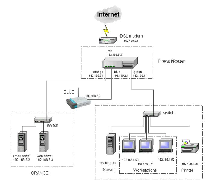
A Linux based firewall/router controls the access to different zones of the system (zones are separate network entities, with no traffic across zones allowed without special permission):
