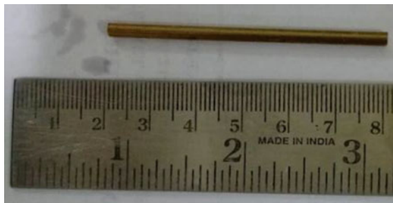
Fig. 22.1 Initial brass tool electrode ( \Phi = 3 mm)
