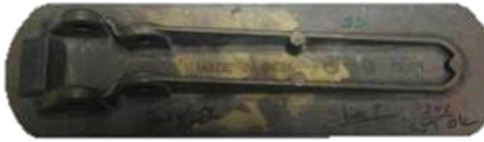
Fig. 47.1 Poor appearance as yellow color patches on the surface of the component
