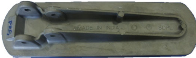
Fig. 47.10 Casting component anodized with low temperature after NSS testing of 1082 h
