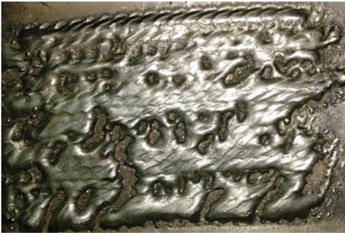
Fig. 49.2 Deposition with irregular weld bead (lower energy and lower powder supplied per unit track)
