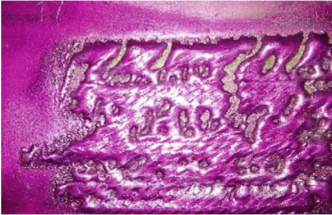
Fig. 49.4 Deposition showing spatter (lower energy, higher speed and higher powder feed rate)
