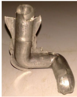
(b) Processed AA6061 aluminium billet after one complete three turn cycle
