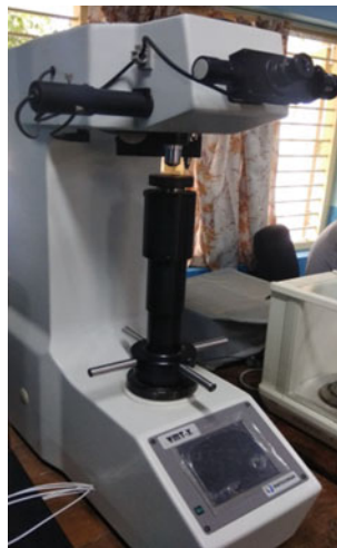
Fig. 15.7 Matsuzawa VMT-X7 for measuring Vickers hardness
