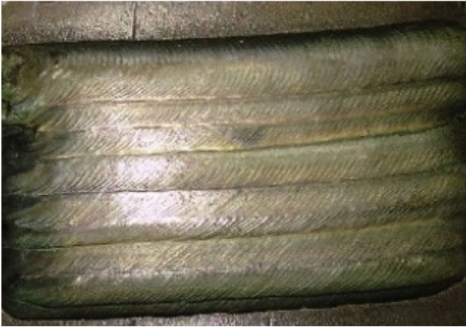
Fig. 49.5 Deposition showing smooth overlapping tracks (appropriate energy and powder)
