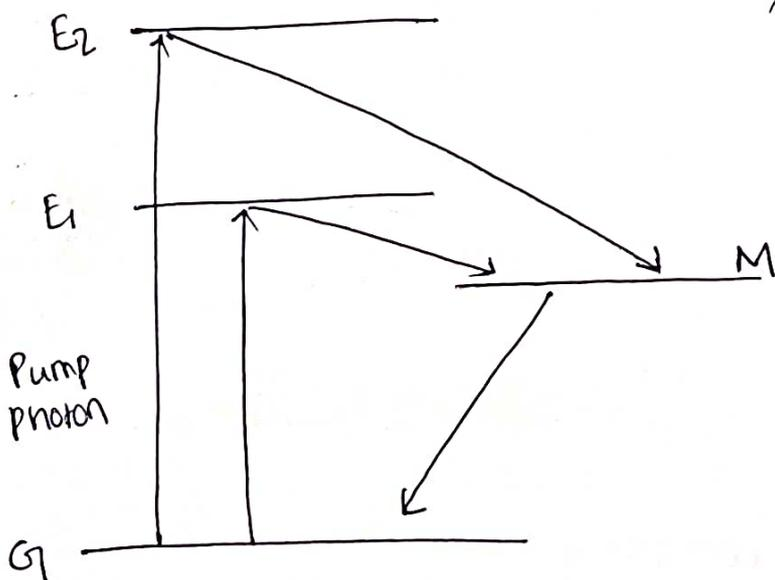
→ The main characteristics of the energy levels of a  $Cr$  ion is the fact that the bands  $E_1$  &  $E_2$  have a lifetime of  $\approx 10^{-8}$  sec whereas the state marked  $M$  has a lifetime of  $\approx 3 \times 10^{-3}$  sec. A state characterized with such a long life is known as metastable state.
