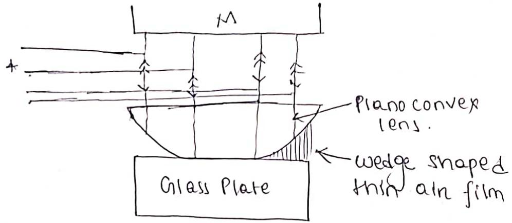
A plano convex lens is placed on a glass plate in such a way that a ~~thin wedge shape~~ its curved surface lies on the glass plate. Then an air film of gradually increasing thickness is formed between the 2 surfaces.
