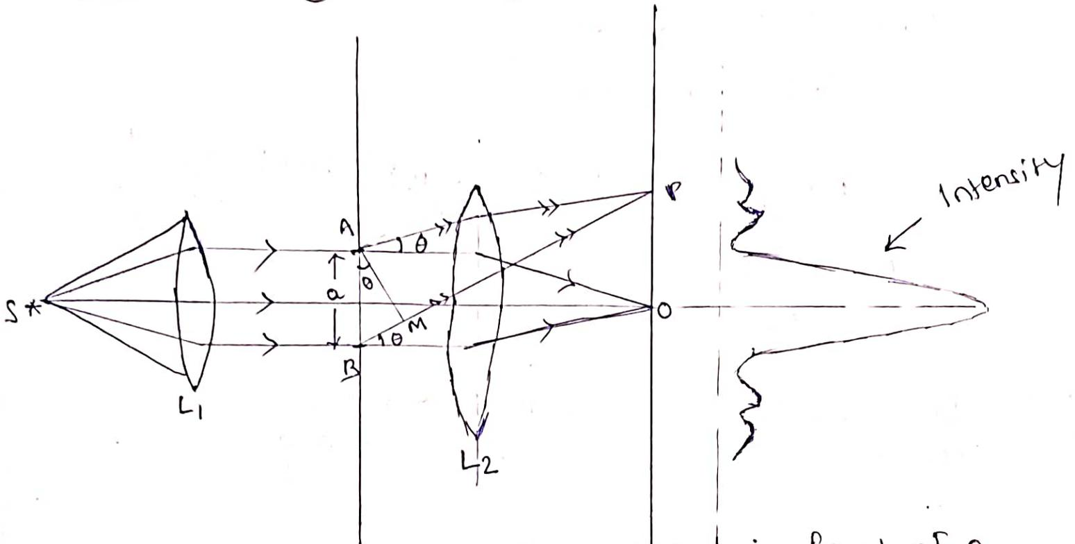
Let a slit  $AB$  of width ' $a$ ' be placed in front of a source ' $S$ '. A beam of monochromatic light of wavelength ' $\lambda$ ' from the source is incident on it through lens  $L_1$ . The diffracted beam from the slit is focussed on the screen with the help of lens  $L_2$ .
