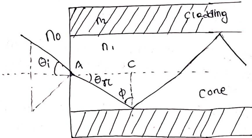
Let a ray enter at an angle ' $\theta_i$ ' from axis & refract at core at angle ' $\theta_r$ '.
