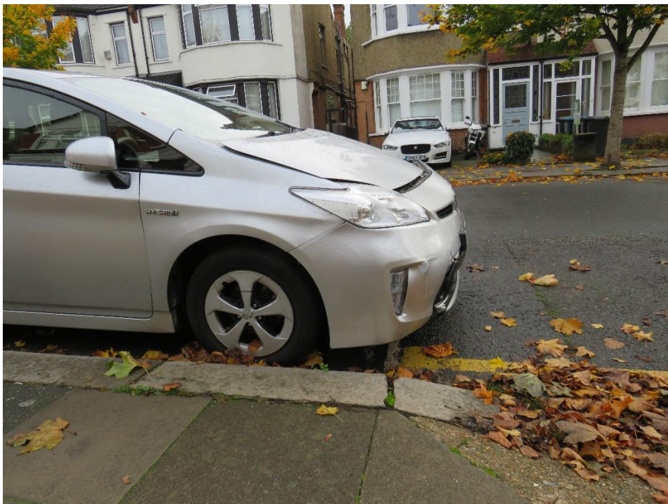
Figure 8 Damage to the Prius includes slightly displacing the whole of the front panel and the bonnet.
