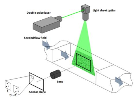
A laser is chosen as the illuminating light source in PIV because laser can deliver high light intensity for very short pulses, which freeze the motion of seeding particle in effect. The particles that are seeded to flow are typically fine TiO2 powers. It is can be assumed that the seeding particles follow the motion of fluid parcels that the seeding particles reside in exactly due to the very small size of the seeding particles.
