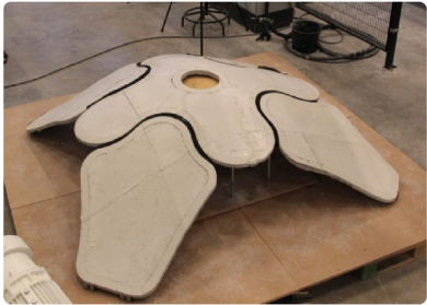
a) a panel, horizontally printed, shell and fill application: TU Delft, Netherlands
