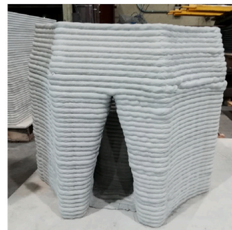
Fig. 20. Printed maximum overhang: (a) front view of layer deposition with maximum overhang of 65^\circ and (b) self-supporting overhang [92].
