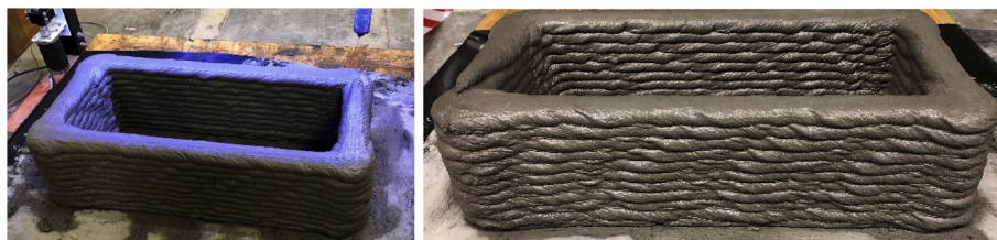
Fig. 5. Rectangular printed concrete section with 15 mm layer height from which 3DPC samples tested were cut.
