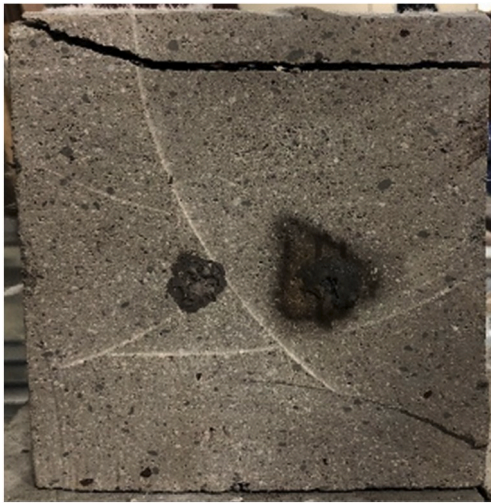
Fig. 26. C3DPC Sample 1 – Interlayer delamination as a result of spalling.
