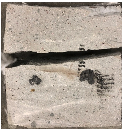
Fig. 28. C3DPC Sample 3 – Interlayer delamination.
