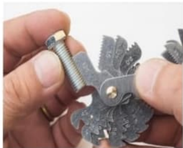
Fig. 3.2 Screw Thread Pitch Measurement using pitch gauge
