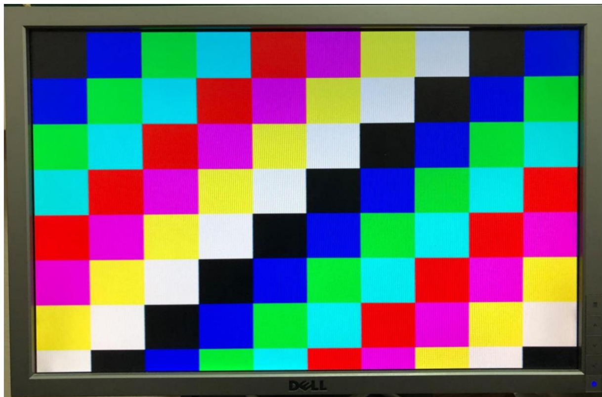
Figure 6. Color Checkerboard test image (each square has dimensions 64x64) for "000" input
