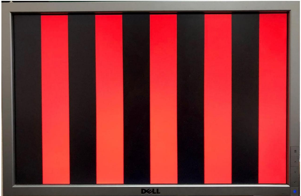
Figure 9. Vertical Red Bars test image (the width of each red bar is 64 lines) for "011" input
