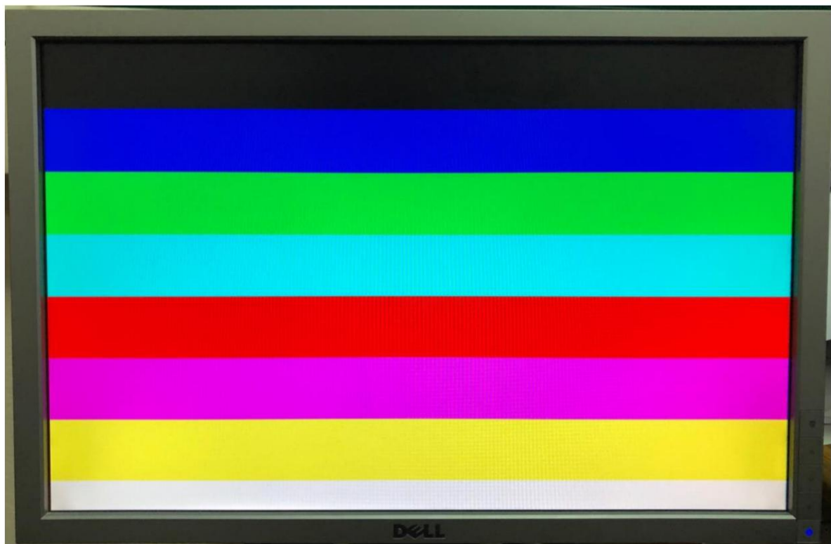
Figure 8. Horizontal Bars test image (the height of each bar is 64 lines) for “010” input
