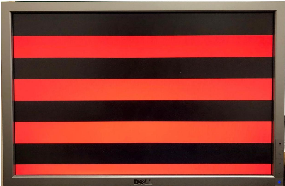
Figure 10. Horizontal Red Bars test image (the height of each red bar is 64 lines) for "100" input
