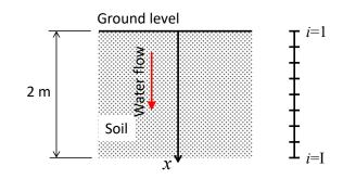
A coordinate *x* is defined and its origin is on the ground level and pointing downwards. The governing equation is the convection diffusion equation
