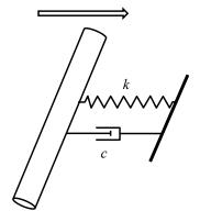
The electricity generator can modelled by a damper that extract energy from the motion of the cylinder with a constant damping constant of c. The structural damping is considered to be negligibly small. Considering the power given by the fluid should be the same as the power received by the damper, the power can also be calculated using the energy received by the electricity generator (damper) as:
